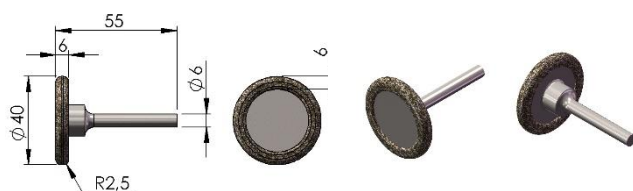
DIA PIN 40x6x6mm D711 114.F05673.0 Länge 55mm
