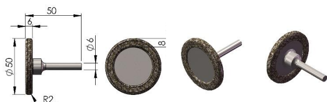
DIA PIN 50x6x6mm D711 114.F01871.0 Länge 50mm
